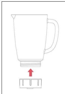
4. Place the glass jar with blade assembly unit interface on the motor unit. The handle can be placed in two positions: either located at the right hand side or left hand side.
