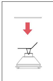
2. Place the blade assembly unit on the interface.
