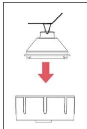
3. Screw the unit interface onto the glass jar bottom until it is fixed properly.
